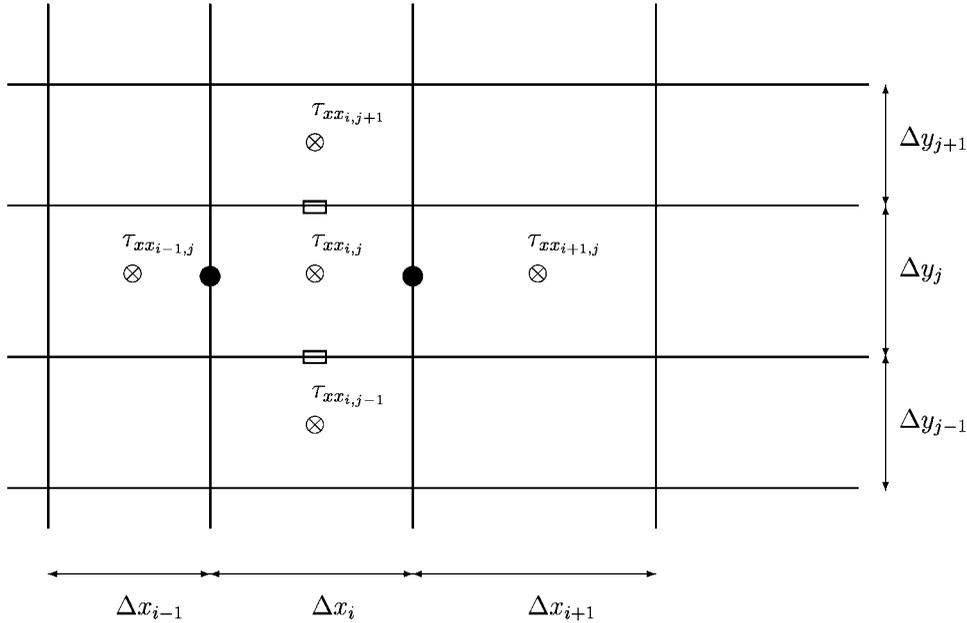
Figure 4. Finite volume discretization for  $\tau_{xx}$ .
